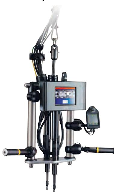
*A vertical two channel Multiple by Express® fixture with QST spindles.*
