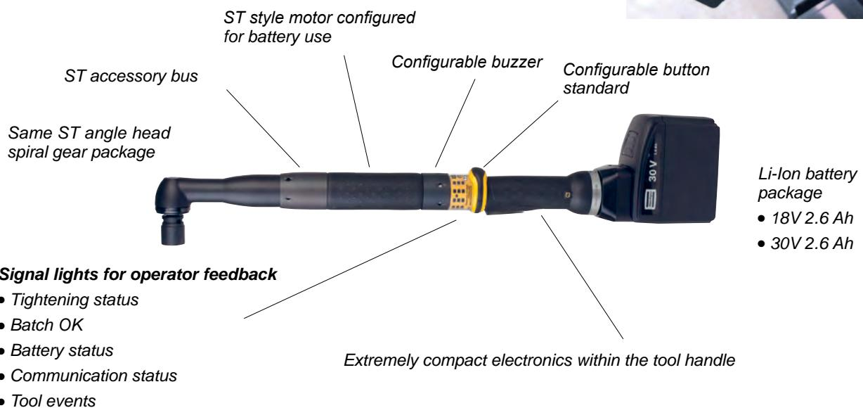
Tensor STB offers genuine ergonomic and flexibility advantages for the operator which, in turn, raises operator efficiency.
