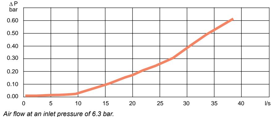
**QIC 10SE and NIP EU 7.6, 22 l/s (recommended air flow at 6.3 bar pressure)**
