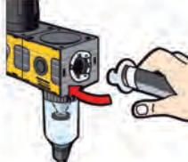
Never open a quick coupling with a screwdriver in order to ventilate the air.
